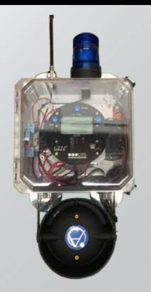
The Gen II WireFree *Relayer* OI-7530 is a wireless relay/alarm system specifically designed for use in conjunction with OTIS Instruments Gen II WireFree products.
